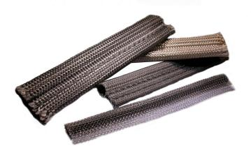
Our tadpole gaskets are designed to provide a high temperature thermal seal in industrial, laboratory, commercial, and residential ovens and dryers with a maximum continuous operating temperature of 1000°F/540°C. Constructed with type E fiberglass, the bulb may be filled with various constructions of either fiberglass or stainless steel in order to achieve the proper design compression.
